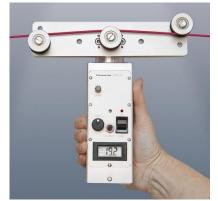
Description: Electronic tensionmeter, battery-operated, for short-time measurement
